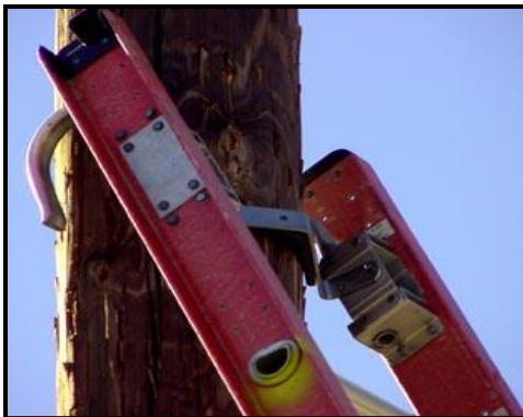
V-Grip supported against pole to prevent turning.
